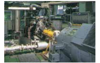
Engine bench setup is used for testing and evaluating next-generation engines with a focus on reducing exhaust gas, enhancing fuel efficiency and boosting quality
